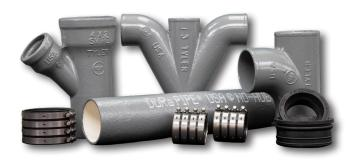
DuRa Pipe™ is an enhanced epoxy coating applied to cast iron soil pipe and fittings made in the U.S.A. DuRaPipe™ is well-suited for aggressive DWV applications where greater performance is required. This is not an equivalent or viable option for acid waste pipe.
